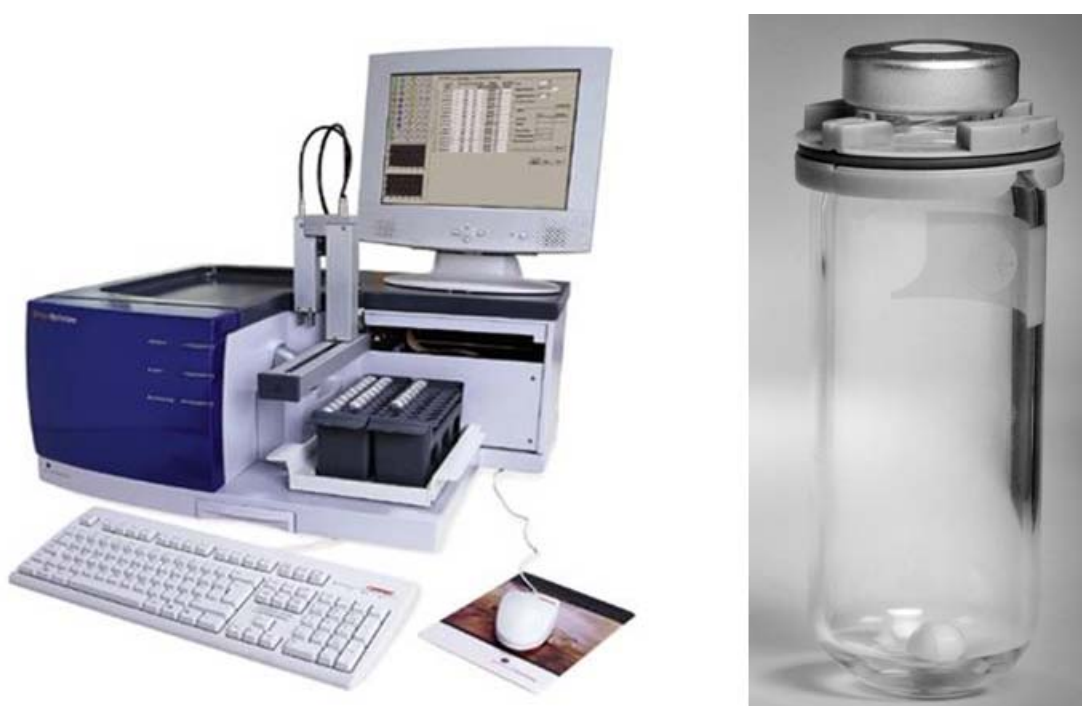
Figure 1. Optimizer Sixty EXP single-mode microwave reactor with 20 mL reaction vessel (Biotage AB, Sweden).
