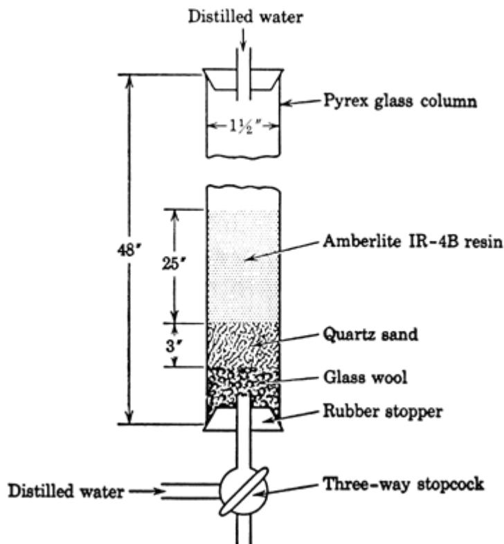
The solid *ε*-aminocaproic acid hydrochloride is dissolved in 1 l. of distilled water. This solution is passed through the column (downflow) and followed by at least 2 l. of distilled water (Note 5).
