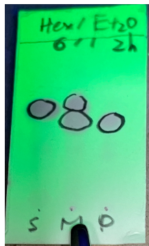
Figure 6. TLC analysis (Note 40); S is starting material ( 2 ), P is product ( 3 ), and M is a co-spot; photo provided by checkers)
