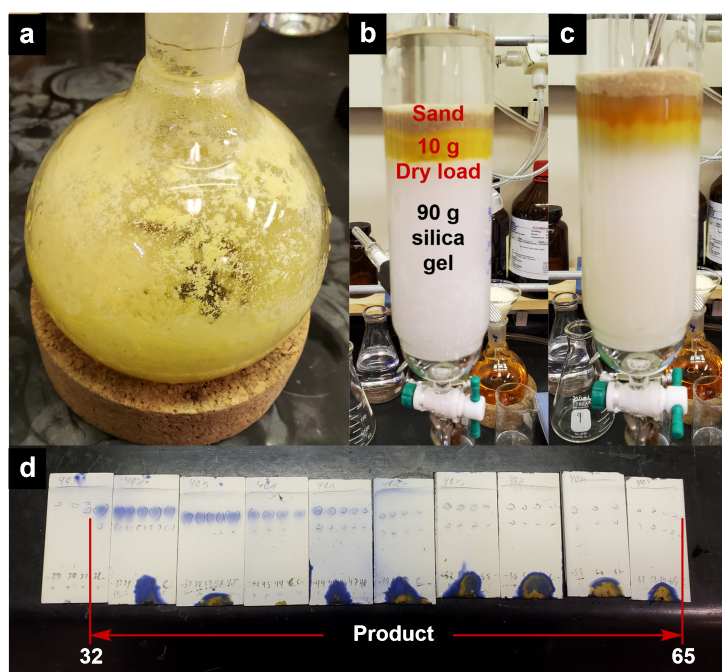
Figure 4. a) Crude filtrate concentrated onto 10 g of silica gel. b) addition of crude mixture on silica followed by sand to pre-equilibrated 90 g silica gel flash column with approximately 100 mL hexanes. c) Appearance of flash column after product had fully eluted. d) Fractions containing product are confirmed by TLC analysis on silica gel with EtOAc-hexane (2: 3 v/v) as eluent and visualizing with both UV and CAM staining. Product 1 is collected in fractions 32 to 65 (photos provided by submitters)
