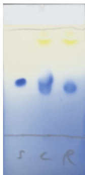
Figure 11. The progress of the reaction is monitored by TLC analysis on silica gel with 2% acetone in \text{CH}_2\text{Cl}_2 as the eluent (Note 25). Spots are visualized after the plate is dipped in ceric ammonium molybdate stain and heated. Note: S = starting material (2), C = co-spot lane, R = reaction mixture containing catalyst ( R_f = 0.86 , yellow spot) and product 3.
