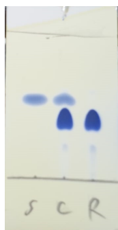
Figure 6. The progress of the reaction is monitored by TLC analysis on silica gel plates using 10% EtOAc in hexanes as the eluent. TLC spots are visualized by staining with ceric ammonium molybdate stain. Note: S = starting material, C = co-spot lane, R= reaction mixture; Compound 1 ( R_f = 0.54), epoxide product 2 ( R_f = 0.42) (Photo provided by checkers)
