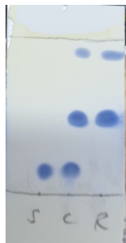
Figure 2. TLC of the crude reaction mixture, stained with ceric ammonium molybdate stain. Mobile phase: 10 % EtOAc in hexanes. Note: S = starting material, C = co-spot lane, R = reaction mixture. Starting material trans -2-hexen-1-ol ( R_f = 0.17 ), product 1 ( R_f = 0.54 ) (Photo provided by checkers)
