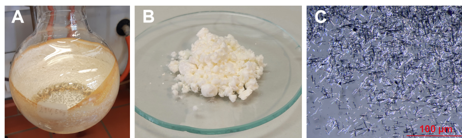
Figure 4. (A) Product 2 after evaporation of column chromatography fractions; (B) Compound 2 after the washings; (C) Compound 2 viewed under a microscope (photos provided by authors)
