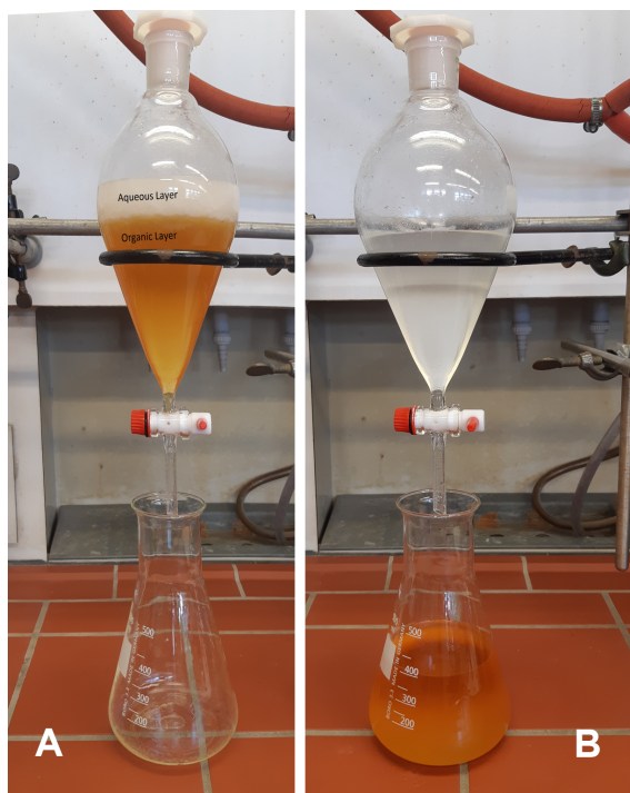
Figure 2. (A) Biphasic mixture after transferring to separatory funnel and shaking; (B) Final extraction of the aqueous phase with \text{CH}_2\text{Cl}_2 (photos provided by authors)
