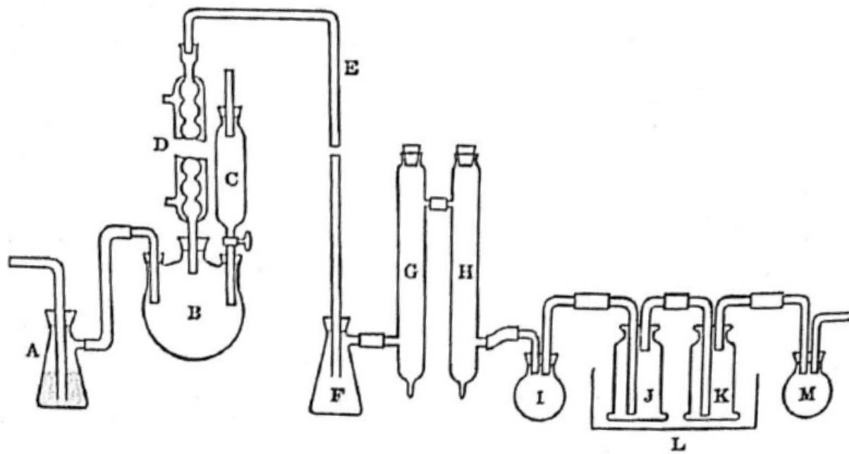
A long (75-cm.) water-cooled bulb condenser *D* is connected to the middle neck of the generator flask *B*. The large bore glass tube *E* connects the top of the condenser *D* with trap
