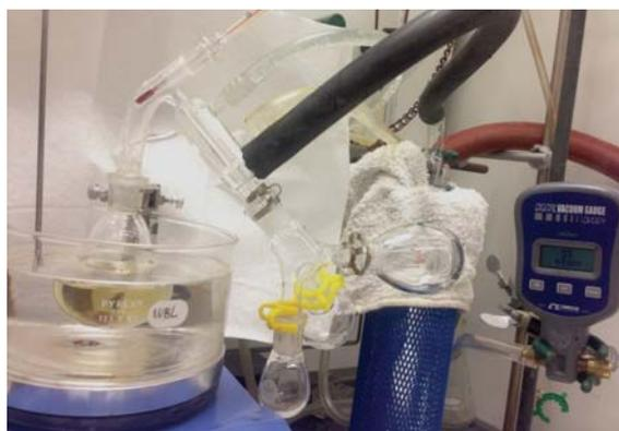
Figure 2. Vacuum distillation apparatus
