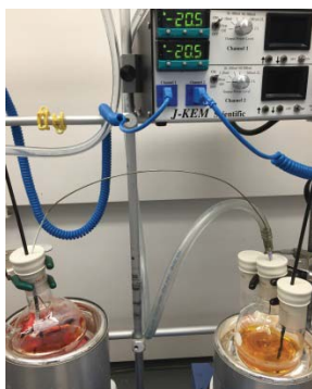
Figure 1. The red solution of deprotonated 2-picoline (left) is transferred via cannula to the solution of \text{TMSCl} (right)
