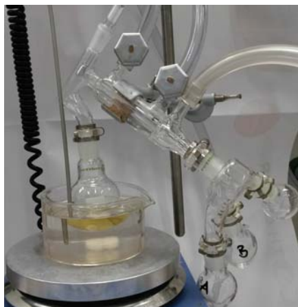
Figure 9: Distillation apparatus for further purification of the product
