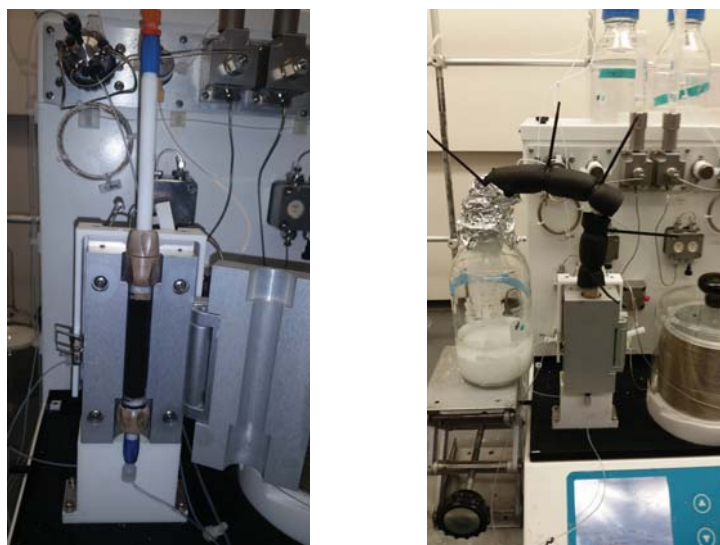
Figure 1. (a) Cartridge that contains the MnO 2 , (b) Uniqsis flow system in operation
