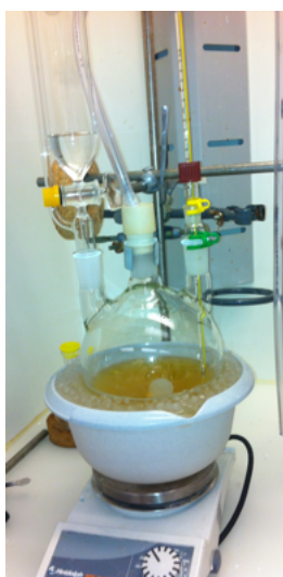
Figure 2. Glassware assembly for the mesylation step (picture obtained from submitters)
