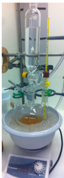
Figure 4. Glassware assembly for the hydrolysis reaction- Step B (picture obtained from submitters)
