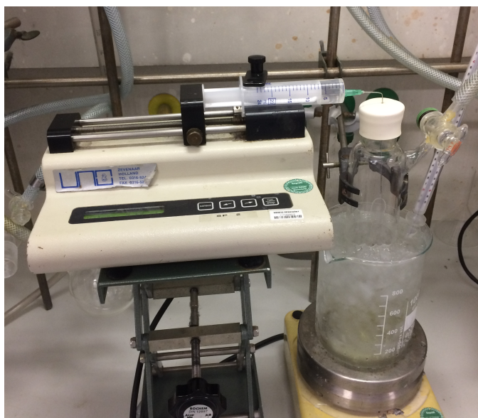
Figure 2. Reaction setup for addition of n -butyllithium (formation of boron ate complex)
