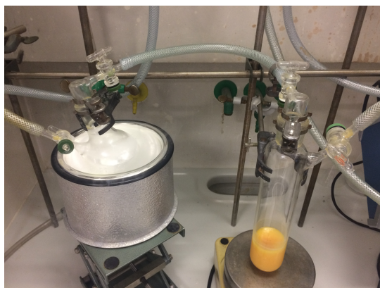
Figure 4. Setup for solvent removal under reduced pressure using a separate cooling trap
