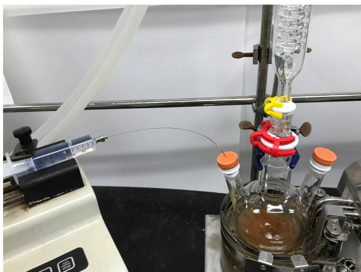
Figure 3. Addition of phenylsilane by syringe pump
