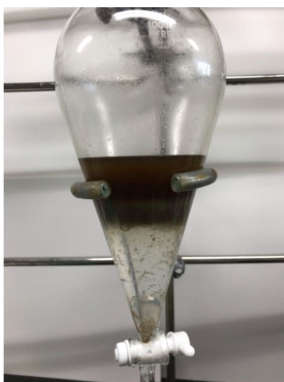
Figure 6. (a) The reaction mixture in separatory funnel after the addition of EtOAc, 1.0 M NaOH, and saturated aqueous sodium chloride (b) The reaction mixture after sitting for 20 min
