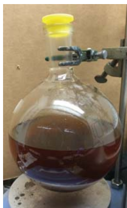
Figure 4. Brown homogenous mixture was formed upon stirring with water and diethyl ether (Photo provided by Submitters)
