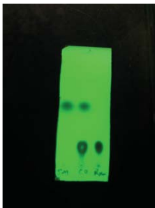
Figure 3. Thin layer chromatography of the crude reaction mixture (left lane = 5-bromopyrimidine, middle lane = cross spots of 5-bromopyrimidine and the reaction mixture, right lane = reaction mixture) (Photo provided by Submitters)
