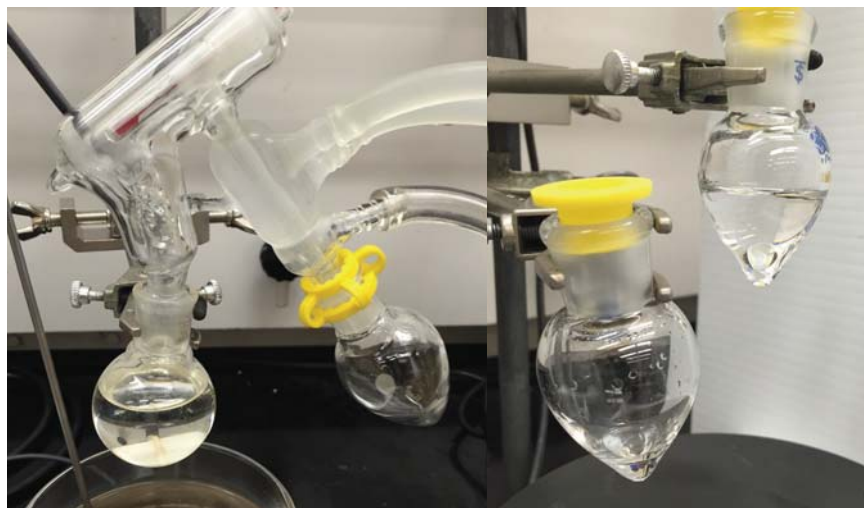
Figure 5. Distillation apparatus and pure final products
