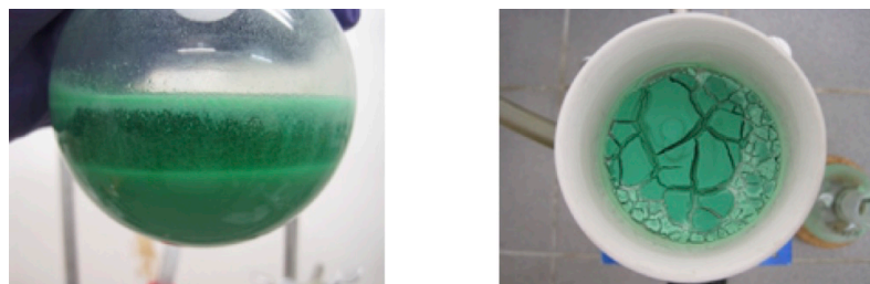
Figure 8. Precipitation in pentane (left) and filtration (right)
