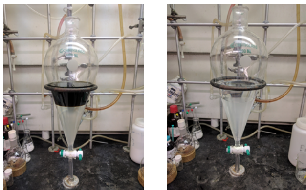
Figure 3. Reaction mixture being quenched with sodium bicarbonate (left) and the final extraction with ethyl acetate (right)
