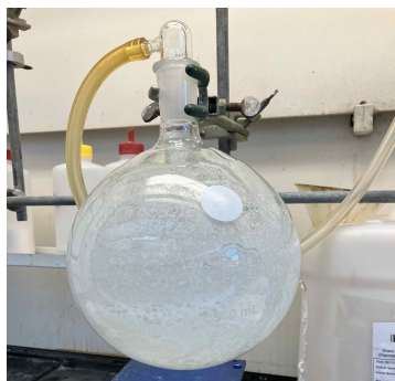
Figure 5. Almost dry (slightly sticky/oily) crude product after acidification and concentration of extracts
