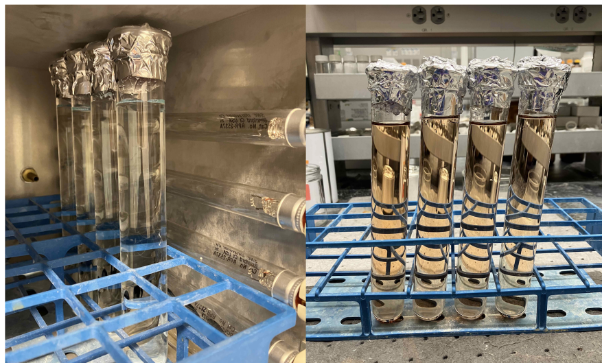
Figure 1. (A) Quartz tubes containing reaction solution in photoreactor prior to irradiation. (B) Quartz tubes after irradiation
