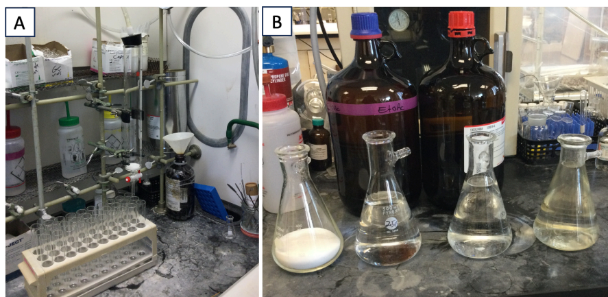
Figure 10. (A) Glass chromatography column positioned above test tube rack; (B) Mobile phases of increasing polarity prepared prior to running the column (photo provided by the authors)
