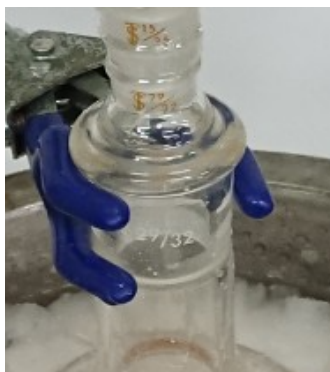
Figure 15. 4-Nitrophenyl chloroformate on the wall of the adaptor (photo provided by Checkers)
