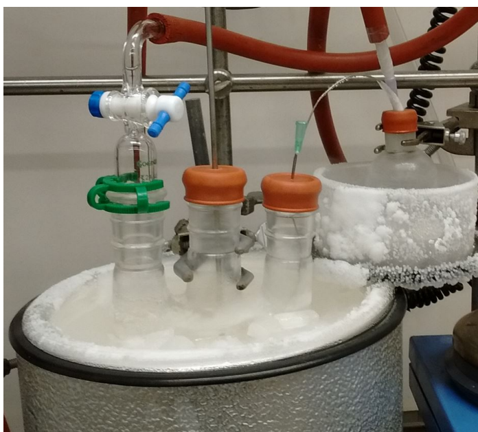
Figure 1. Reaction assembly for step A (photo provided by submitters)
