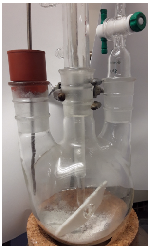
Figure 5. Reaction assembly for organocopper compound formation (photo provided by checkers)
