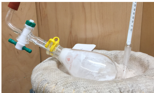
Figure 13. Drying powdered 4 Å molecular sieves (photo provided by submitters)
