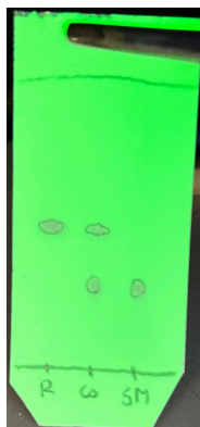
Figure 7. TLC of the crude reaction mixture after 2 h (SM = 1-(3-chloro-4-hydroxyphenyl) ethan-1-one starting material, Co = co-spot of S and R, and R = reaction mixture) (photo provided by checkers)
