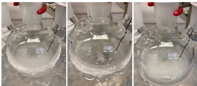
Figure 6. (A) Reaction mixture immediately after placing into an ice bath; (B) Reaction mixture becomes homogeneous solution when internal temperature reached -14\text{ }^{\circ}\text{C} ; (C) Reaction mixture turns back into heterogeneous slurry while stirring at 0\text{ }^{\circ}\text{C} (photos provided by checkers)
