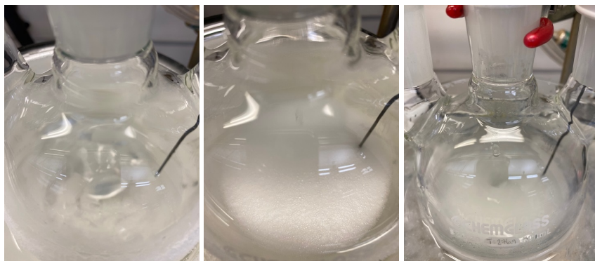
Figure 2. Reaction mixture (A) after DIBAL-H addition; (B) Effervescence during methanol addition; (C) White precipitate at 0 °C (photos provided by checkers)
