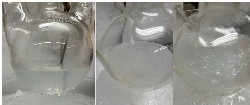
Figure 7. Reaction mixture turned into a gel after warming to 0 °C when stirring is insufficient. (A) Mixture side view; (B) Mixture top view; (C) Mixture after mechanically broken up using a metal spatula (photos provided by authors)
