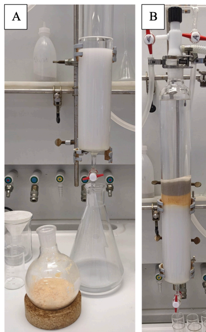
Figure 8. (A) Preparation of column and crude material; (B) Loaded column (Photos provided by authors)
