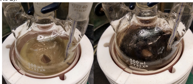
Figure 3. Reaction mixture at 90 °C before (left) and after (right) adding the \text{BrCF}_2\text{CO}_2\text{K} /DMF solution
