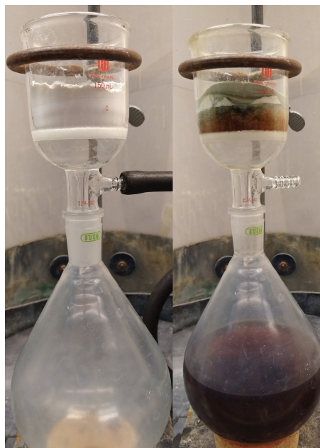
Figure 5. Silica plug before (left) and after (right) filtration
