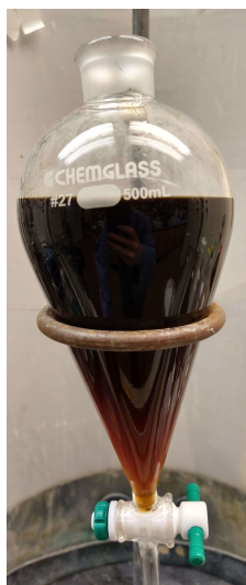
Figure 4. Separatory funnel after transferring the organic and aqueous layers from the 500-mL reaction flask
