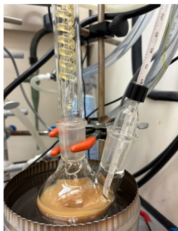
Figure 14. The refluxing setup (photo provided by checkers)
