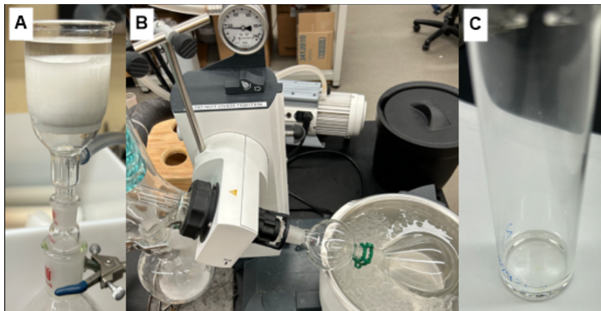
Figure 16. Glassware used for purification and rotary evaporator configuration; A. filtration of diyne 4 and pentane through silica gel pad; B. evaporation setup for removing pentane from diyne 4 ; C. physical appearance of diyne 4 (photos provided by authors)
