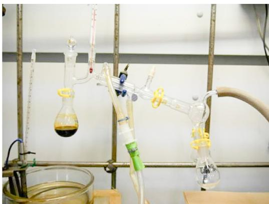
Figure 10. Apparatus assembly for distillation
