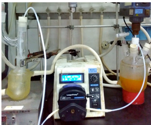
Figure 12. Addition of UHP solution under thermal insulation (Photos provided by submitters)
